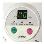
If pressing button, the move mode moves in order of mode A, mode B, mode A+B.
